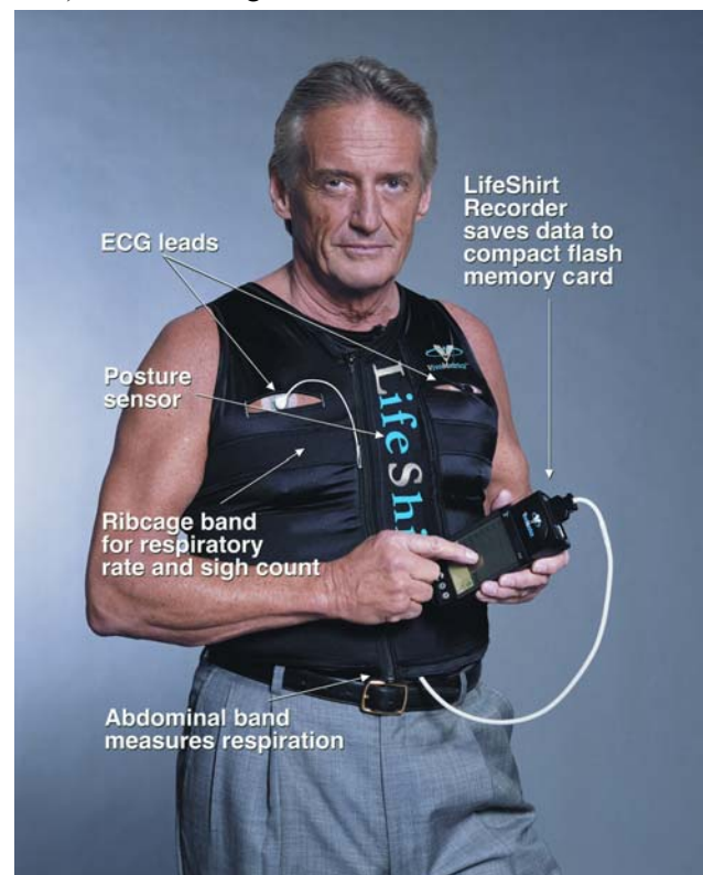
Figure 1. LifeShirt System (Courtesy of VivoMetrics).
